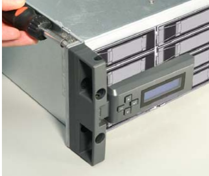
Figure 4. Attach the LCD panel to the VessRAID enclosure
