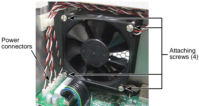
Figure 4. RAID Controller cooling fan
