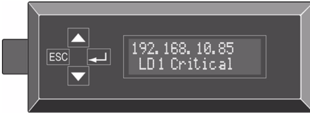
Figure 10. The optional LCD panel reports a Critical logical drive
